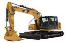
Excavators (hydraulic) are heavy construction equipment consisting of a boom,dipper (or stick), bucket and cab on a rotating platform known as the "house". Thehouse
